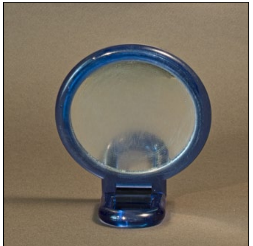
An inexpensive plastic double-sided hand mirror is a valuable assistant for reflecting light on a subject. Sand down one side so it is opaque (as shown here) and get very gently light when you need it.
